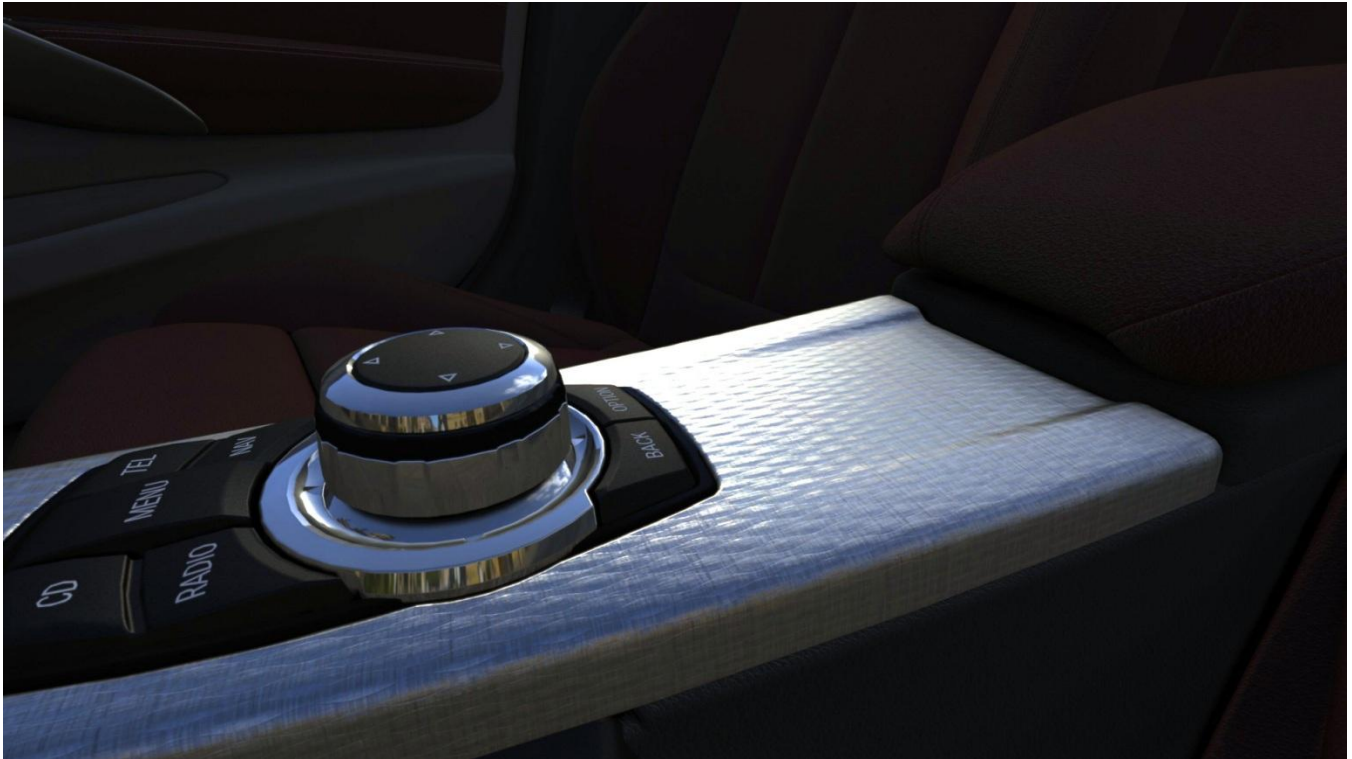
3D Car Model Rendered with Five Different Measured Anisotropic Metal Materials for the Radio Control Panel
