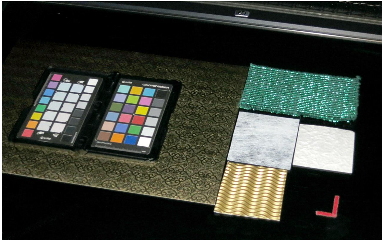
Another set of materials in the scanner Including (under the ColorChecker chart) a Flower-Gold material with spatially varying specular roughness.
